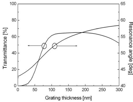
Fig. 2. Transmission characteristics of a transmission-type SPR structure with a dielectric grating. The effects of the grating thickness on the transmittance efficiency (1T) and the resonance angles are shown. The silver metal film thickness is  $d_m = 40$  nm. The dielectric grating has a period of  $\Lambda = 600$  nm and  $f = 0.5$ .
