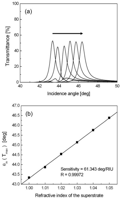
Fig. 7. (a) Transmittance and (b) linear regression analysis between resonance angle and superstrate refractive index of a transmission-type SPR sensor with a metallic grating at  $d_g = 24$  nm in air. As the refractive index of the superstrate increases, the transmittance peak shifts from  $43.34^\circ$  to  $46.38^\circ$ .
