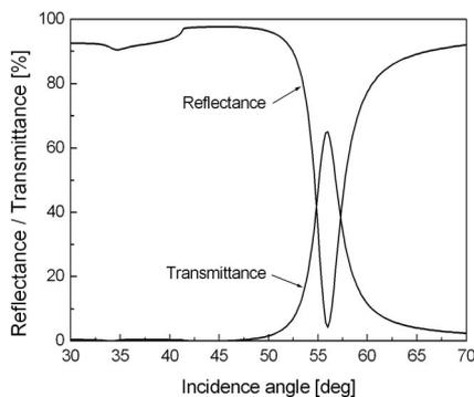
Fig. 3. Calculated reflectance and transmittance curves (1T) for a dielectric grating as a function of incidence angle. The grating thickness is  $d_g = 180$  nm. At  $\theta_{\text{in}} = 55.92^\circ$ ,  $T_{\max} = 65.28\%$ .
