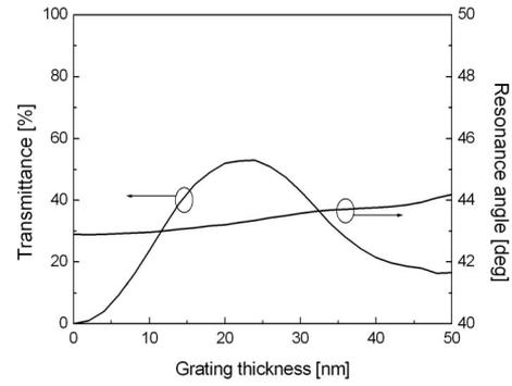
Fig. 4. Transmission characteristics of a transmission-type SPR structure with a metallic grating. The effects of the grating thickness on the transmittance efficiency (1T) and the resonance angles are shown. The silver metal film thickness is  $d_m = 40$  nm. The silver metal grating has a period of  $\Lambda = 600$  nm and  $f = 0.5$ .
