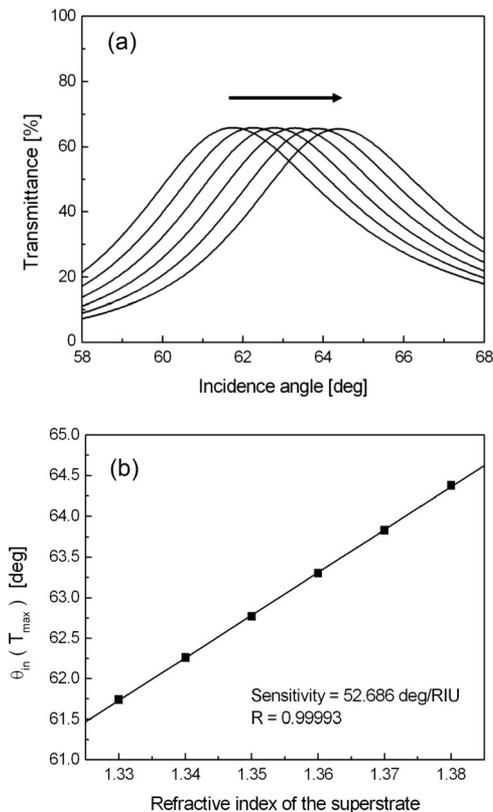
Fig. 8. (a) Transmittance and (b) linear regression analysis between resonance angle and superstrate refractive index of a transmission-type SPR sensor with a dielectric grating at  $d_g = 80 \text{ nm}$  in water. As the refractive index of the superstrate increases from 1.33 to 1.38 in steps of 0.01, the transmittance peak shifts from  $61.74^\circ$  to  $64.38^\circ$  in the direction of the arrow.
