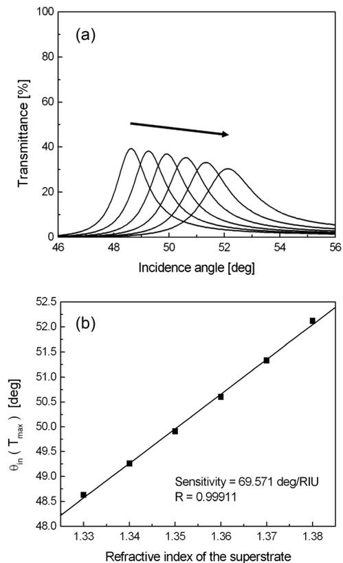
Fig. 9. (a) Transmittance and (b) linear regression analysis between resonance angle and superstrate refractive index of a transmission-type SPR sensor with a metallic grating at  $d_g = 22 \text{ nm}$  in water. As the refractive index of the superstrate increases, the transmittance peak shifts from  $48.63^\circ$  to  $52.12^\circ$ .
