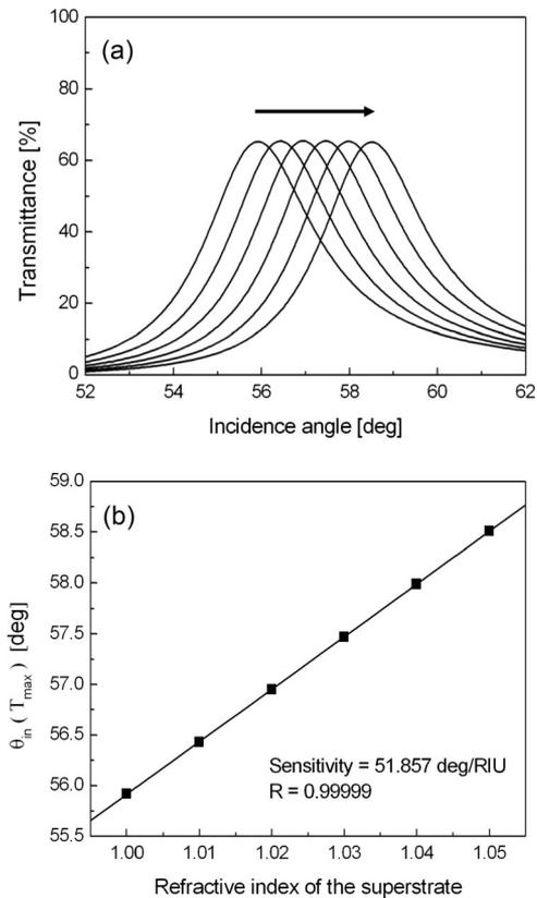
Fig. 6. (a) Transmittance and (b) linear regression analysis between resonance angle and superstrate refractive index of a transmission-type SPR sensor with a dielectric grating at  $d_g = 180$  nm in air. As the refractive index of the superstrate increases from 1.00 to 1.05 in steps of 0.01, the transmittance peak shifts from  $55.92^\circ$  to  $58.51^\circ$  in the direction of the arrow.  $\theta_{in}(T_{max})$  denotes the incidence angle at maximum transmittance.
