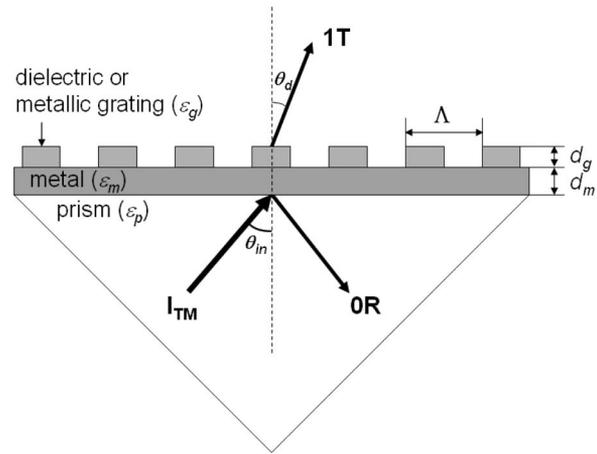
Fig. 1. Schematic diagram of a transmission-type SPR configuration with dielectric or metallic gratings. A thin metal film with a thickness of  $d_m$  is deposited on a prism substrate. Dielectric or metallic gratings with a period  $\Lambda$  and a fill factor  $f$  are regularly patterned on the metal layer. TM-polarized light is incident through the prism substrate at a fixed wavelength of  $\lambda = 633$  nm. The diffracted light transmits into a superstrate environment (air or water).
