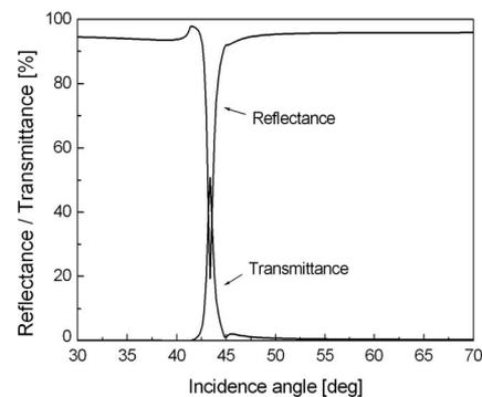
Fig. 5. Calculated reflectance and transmittance curves (1T) for a dielectric grating as a function of incidence angle. The grating thickness is  $d_g = 24$  nm. At  $\theta_{\text{in}} = 43.34^\circ$ ,  $T_{\max} = 52.97\%$ .
