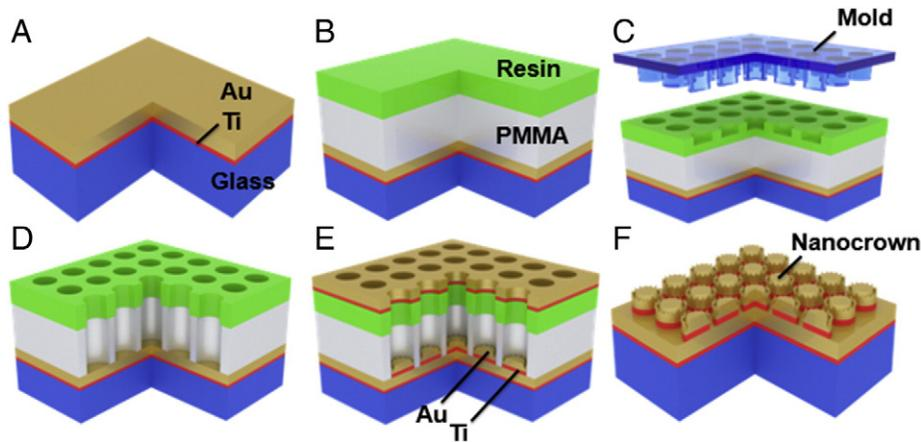
**Fig. 1.** Fabrication procedure of gold nanocrown arrays using UV-NIL and tilted evaporation. (A) Evaporating titanium and gold on a glass substrate, (B) spin-coating PMMA and imprint resin, (C) imprinting gold nanocrown array patterns, (D) etching imprint resin and PMMA, (E) depositing titanium and gold by tilted evaporation technique, and (F) lifting off the resin and PMMA.
