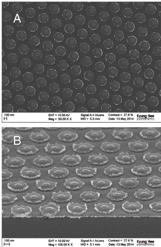
**Fig. 2.** (A) Top-view and (B) side-view FE-SEM images of gold nanocrown arrays with a diameter of 380 nm, height of 50 nm, and pitch of 520 nm. The total pattern area has a size of 15 × 15 mm<sup>2</sup>.
