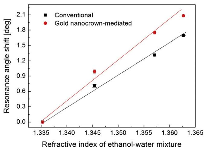
Fig. 4. Resonance angle shift according to a change in bulk refractive index of ethanol-water mixtures for the fabricated SPR samples with and without gold nanocrown arrays. The black and red lines indicate linear fits of experimental results.
