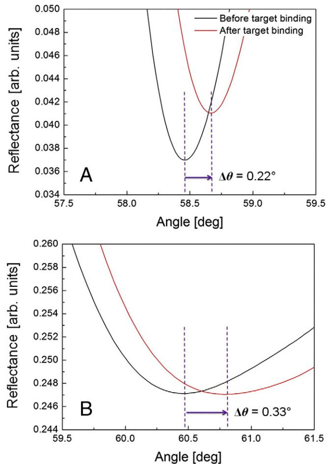
**Fig. 3.** SPR curves obtained from biotin–streptavidin interactions for (A) a thin gold substrate and (B) gold nanocrown arrays on a gold film. The black and red lines represent the results before and after injecting streptavidin biomolecules, respectively.
