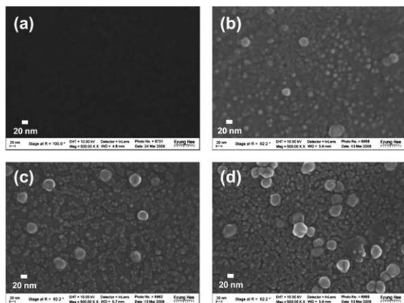
**Fig. 1** SEM images of the gold films after treatment with SPION suspensions at (a) 0.0, (b) 0.5, (c) 1.0, and (d) 2.0 mg ml<sup>-1</sup> concentration.
