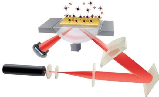
**Fig. 10** Schematics of the optical measurement set-up and the SPR sensor chip.
