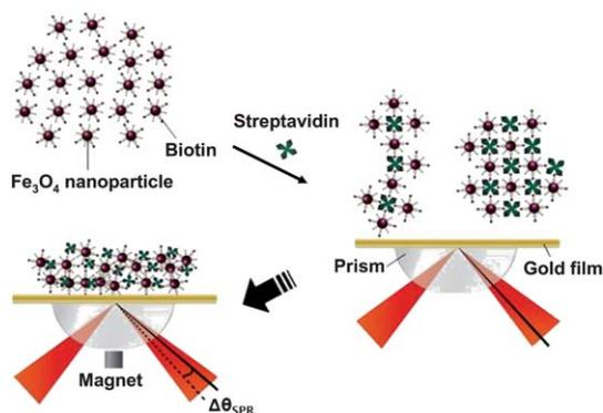
**Scheme 1** SPR detection based on SPIONs and magnetic field.
