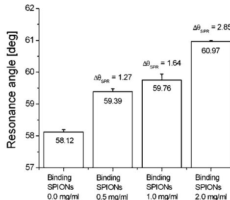
**Fig. 2** Measurement of resonance angles after treatment with the SPION suspensions of concentrations at 0.0, 0.5, 1.0, and 2.0 mg ml<sup>-1</sup>, respectively.
