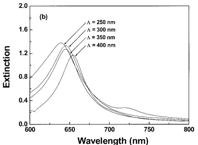
Fig. 2. Extinction spectra of nanowire arrays with a rectangular profile assuming no analytes. For (a) silver and (b) gold nanowires,  $\lambda_{\text{LSPR}} = 562$  nm (silver) versus 645 nm (gold) at  $\Lambda = 350$  nm. The peak extinction and its width (full width at half-maximum) are 1.623 and 36 nm (silver) versus 1.272 and 52 nm (gold).
