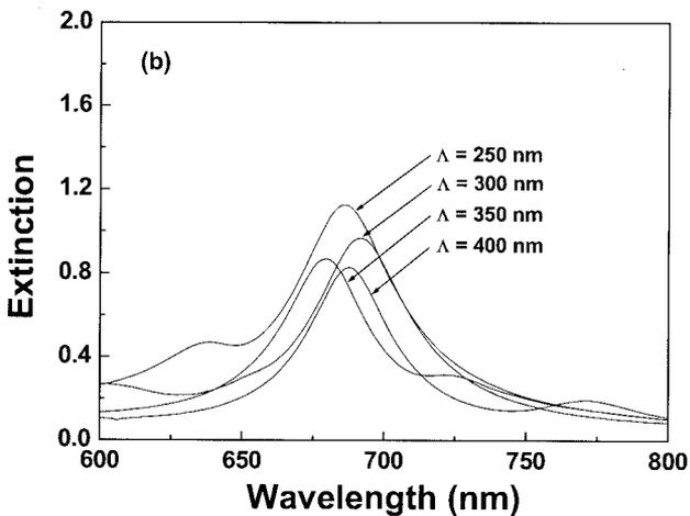
Fig. 6. Extinction spectra of nanowire arrays with an inverse T-profile assuming no analytes. For (a) silver and (b) gold nanowires,  $\lambda_{\text{LSPR}} = 589$  nm (silver) versus 679 nm (gold) at  $\Lambda = 350$  nm. The peak extinction and its width (FWHM) are 1.214 and 38 nm (silver) versus 0.868 and 42 nm (gold).
