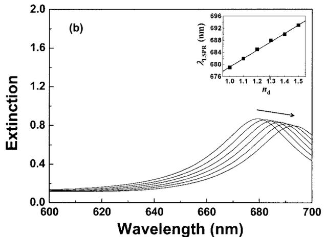
Fig. 7. Extinction spectra of (a) silver and (b) gold nanowires of an inverse T-profile at  $\Lambda = 350$  nm as  $n_d$  increases from 1.0 to 1.5 (increase is in the direction of the arrow). The inset shows linear regression analysis between  $n_d$  and  $\lambda_{\text{LSPR}}$ .
