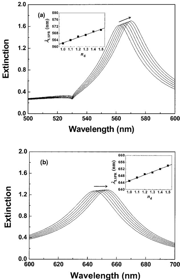
Fig. 3. Extinction spectra of rectangular nanowires of (a) silver and (b) gold at  $\Lambda = 350$  nm as  $n_d$  increases from 1.0 to 1.5 (increase is in the direction of the arrow). The inset shows linear regression analysis between  $n_d$  and  $\lambda_{\text{LSPR}}$ .
