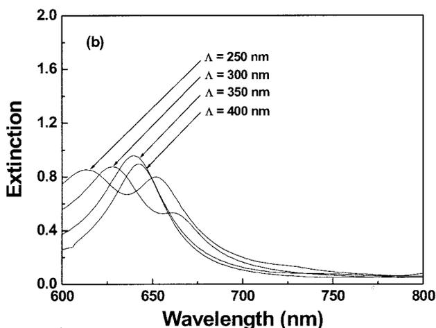
Fig. 4. Extinction spectra of nanowire arrays with a T-profile assuming no analytes. For (a) silver and (b) gold nanowires,  $\lambda_{\text{LSPR}} = 546$  nm (silver) versus 640 nm (gold) at  $\Lambda = 350$  nm. The peak extinction and its width (FWHM) are 1.206 and 33 nm (silver) versus 0.957 and 49 nm (gold).
