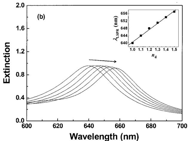
Fig. 5. Extinction spectra of (a) silver and (b) gold nanowires of a T-profile at  $\Lambda = 350$  nm as  $n_d$  increases from 1.0 to 1.5 (increase is in the direction of the arrow). The inset shows linear regression analysis between  $n_d$  and  $\lambda_{\text{LSPR}}$ .
