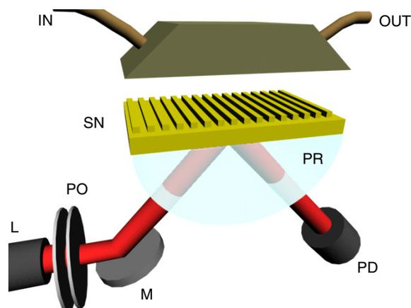
**Figure 2.** Schematics of the optical set-up and the mount of an LSPR assay (IN: inlet, L: laser, M: mirror, OUT: outlet, PD: photodetector, PO: polarizer, PR: prism, and SN: surface nanograting; not scaled).
