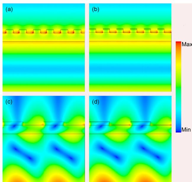
**Figure 6.** Field profiles ( $|H_y|$ ) calculated by the FDTD method: (a) no SAM and (b) with a MUA SAM at  $\Lambda = 60$  nm and same with (c) and (d) at  $\Lambda = 200$  nm.
