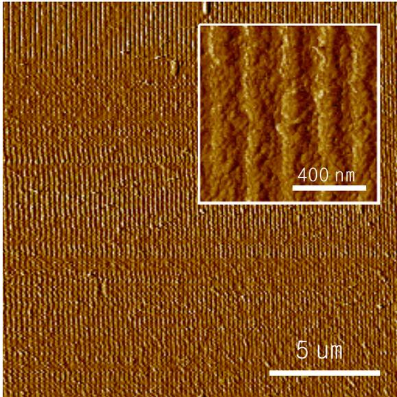
**Figure 3.** Atomic force microscope (AFM) image of dsDNA on a nanograting sample of  $\Lambda = 200$  nm.
