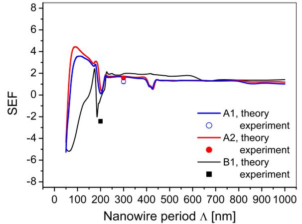
**Figure 4.** Sensitivity enhancement numerically calculated (lines) and experimentally obtained with the various nanograting listed in table 1 (symbols).
