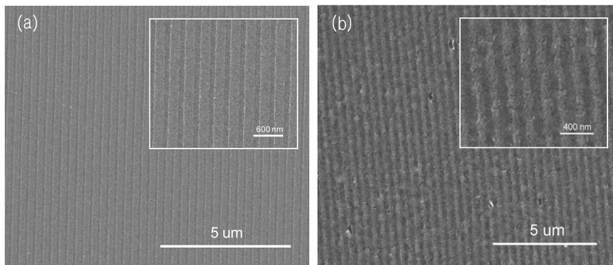
**Figure 1.** Scanning electron microscope image of the fabricated nanograting (a) A and (b) B. The inset shows a magnified image.
