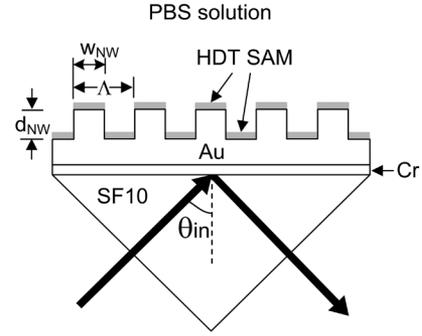
Fig. 1. Schematic diagram of a SPR imaging configuration with periodic gold nanowires. A TM-polarized light with  $\lambda = 633 \text{ nm}$  is incident at an angle  $\theta_{\text{in}}$ . A 40-nm-thick gold film is deposited on an SF10 prism substrate with an attachment chromium layer. Gold nanowires (period:  $\Lambda$ , width:  $w_{\text{NW}}$  and thickness:  $d_{\text{NW}}$ ) are regularly patterned on the gold film. Binding analytes are modeled as a 1-nm-thick HDT SAM in PBS solution.
