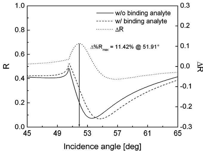
Fig. 3. SPR curves for a nanowire-mediated SPR imaging structure at nanowire period  $\Lambda = 50$  nm,  $VF = 0.1$ , and  $d_{NW} = 20$  nm. The dashed and solid lines represent with and without binding analytes with resonance angles at  $54.63^\circ$  and  $53.58^\circ$ , respectively. The dotted curve is the difference ( $\Delta R$ ) between the SPR curves with and without analytes with a maximum at  $11.42\%$  at  $\theta_{in} = 51.91^\circ$ .
