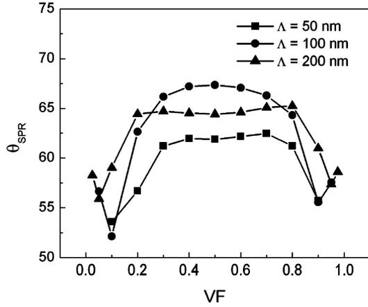
Fig. 5. Resonance angles with VF for nanowires at  $\Lambda = 50$  nm (squares), 100 nm (circles), and 200 nm (triangles).
