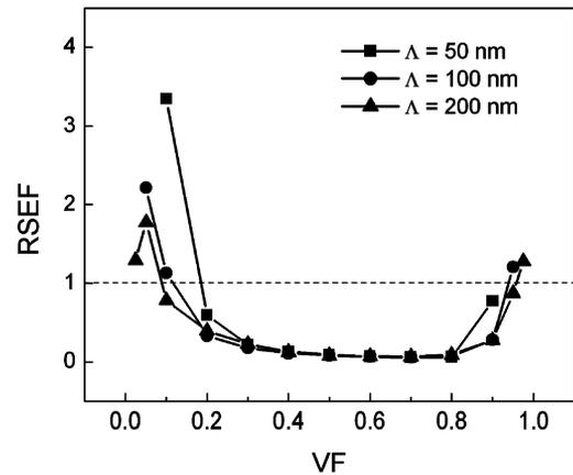
Fig. 4. RSEF characteristics with VF for nanowires at  $\Lambda = 50$  nm (squares),  $100$  nm (circles), and  $200$  nm (triangles). VF varies from  $0$  to  $1$ . The dotted line presents the relative sensitivity based on reflectance for a conventional SPR imaging structure.
