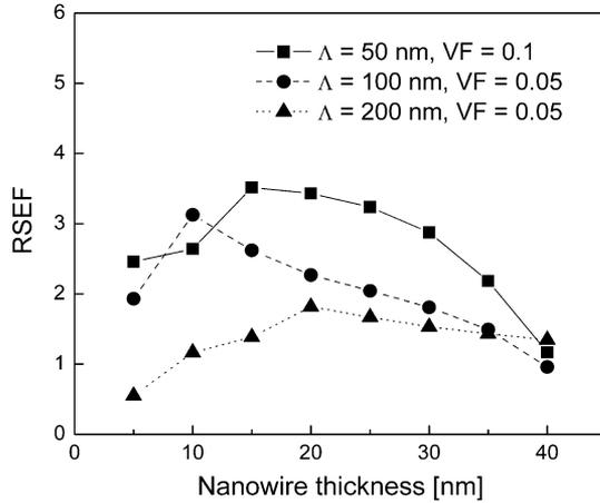
Fig. 7. RSEF characteristics with nanowire thickness  $d_{NW}$  varying from 5 nm to 40 nm with a step of 5 nm. The RSEF reaches a maximum of 3.44 at  $d_{NW} = 15$  nm for  $\Lambda = 50$  nm (squares), 3.05 at  $d_{NW} = 10$  nm for  $\Lambda = 100$  nm (circles), and 1.77 at  $d_{NW} = 20$  nm for  $\Lambda = 200$  nm (triangles).
