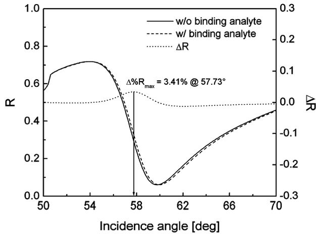
Fig. 2. SPR curves for a conventional SPR imaging structure. The dashed and solid lines represent with and without binding analytes and the resonance angles are  $59.94^\circ$  and  $59.75^\circ$ , respectively. The dotted curve is the difference ( $\Delta R$ ) between the SPR curves with and without analytes with a maximum at  $3.41\%$  at  $\theta_{in} = 57.73^\circ$ .
