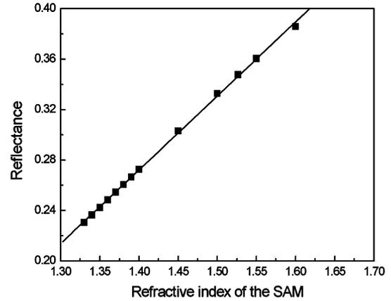
Fig. 8. Linear regression analysis between reflectance and refractive index of a 1-nm-thick SAM in PBS solution. As the refractive index increases from 1.33 to 1.60, the percent reflectance shifts from 23.05% to 38.59% linearly. The correlation coefficient  $R$  is equal to 0.99966.
